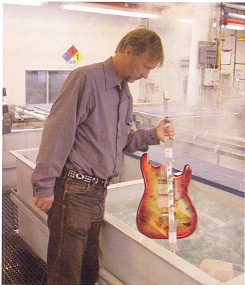
Owner Peter Kellett stands beside one of P.K.'s nine anodizer tanks. The company offers customers superior color quality and thick, hard coatings on Type II and III anodizing.
